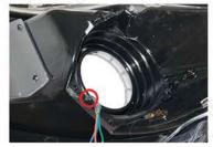
E) Here is an image showing the wires routing through the back of the projector housing. Be sure to route the wires first before installing the halo.
