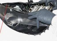
B) Begin seperating the headlight lens and projector bezel from the headlight housing using a Phillips Screwdriver. Pry through the sealant until the two pieces begin to seperate. This step may be difficult, take your time.
