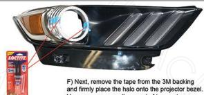
and firmly place the halo onto the projector bezel You may use a small amount of two part epoxy. See image above for epoxy placement.
